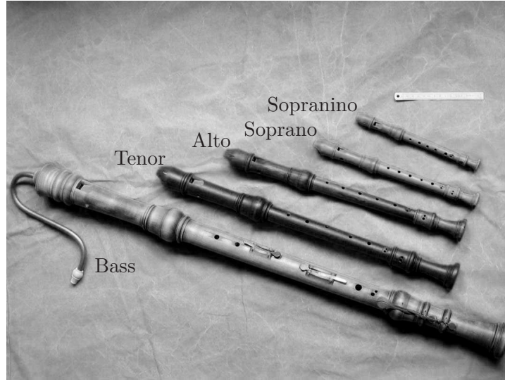
FIG. 7.2: Photography of the five recorders studied. With the bass recorder, the player blows in a bocal, through the “S”-shaped pipe. In the experiments, the instrument is blown directly from the flow channel entrance.
