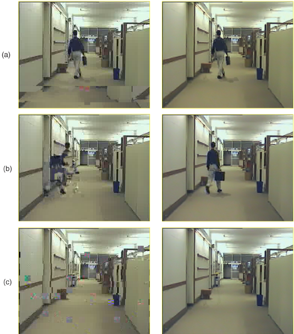
Fig. 8. The tenth, 48th, and 59th images of the sequence “Hall” (COST-211 European project) encoded using MPEG-1 (256 kb/s, 25 f/s) with simulated transmission losses. (Left) standard decoding and (right) proposed decoding.
