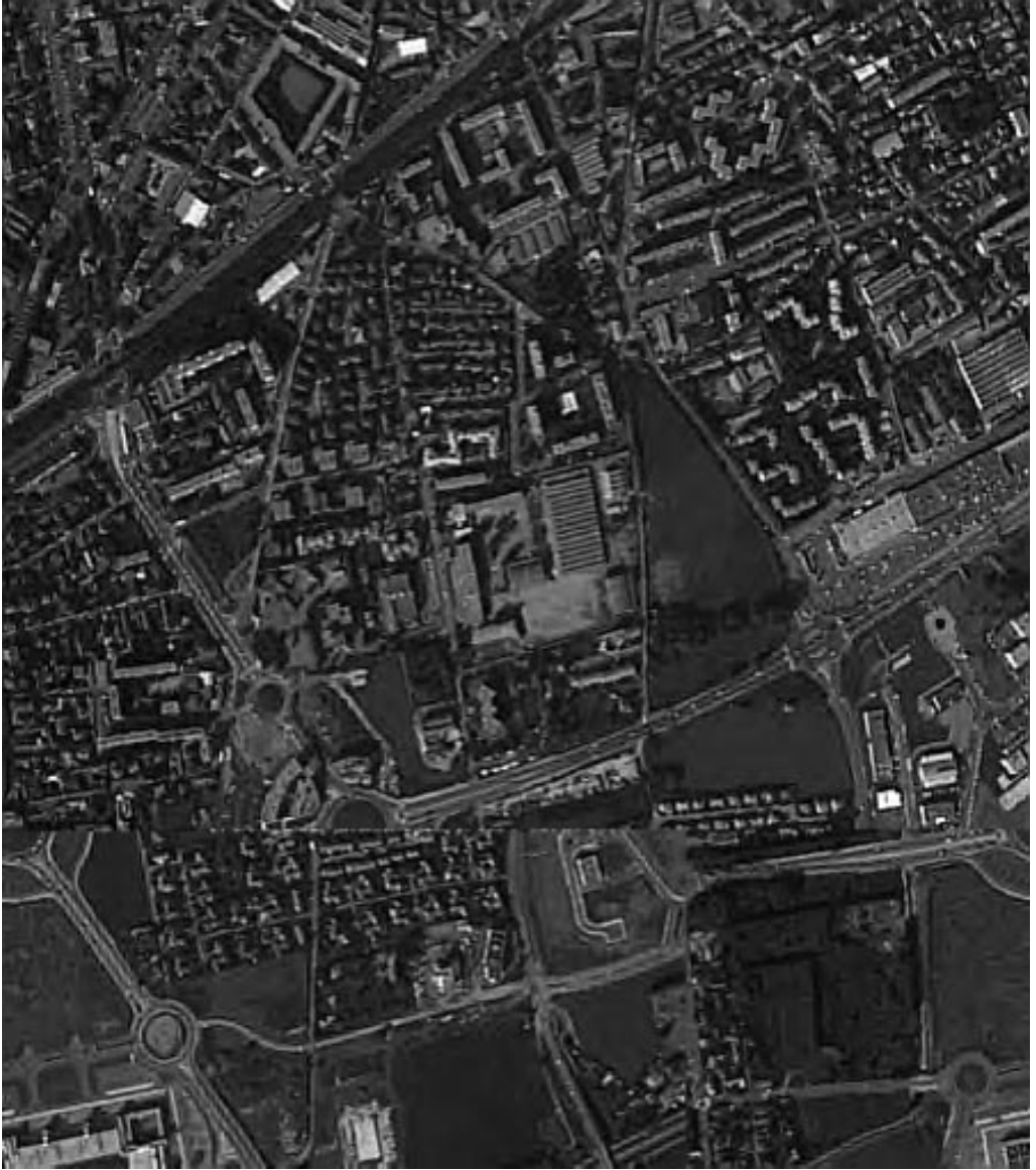
Fig. 6. Image “Nimes” coded on 1.08 bpp (compression ratio of about 7.40 : 1) using wavelet LVQ, with \mathbb{Z}^8 lattice and bit allocation based on exact distortion-rate models. The wavelet coefficients’ pdf is modeled as a Laplacian. Peak SNR = 37.09 dB.
