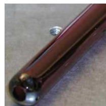
Fig. 2. (b) chalcogenide tube formed by rotational casting
