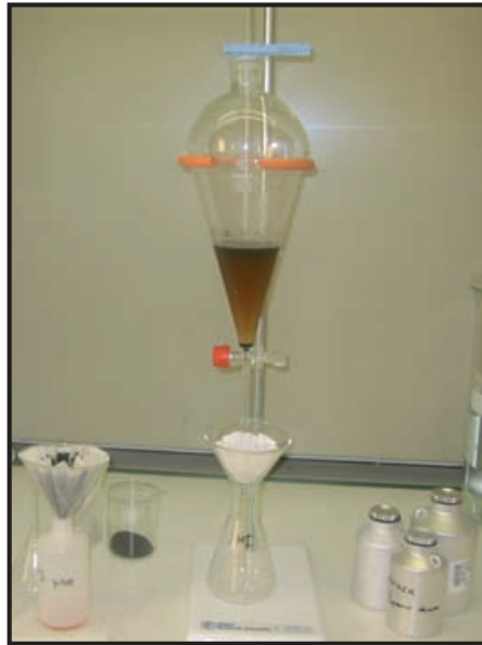
Figure 2.7: Set-up for mineral separation with heavy liquids. The heavy liquid used here is methylene iodide.
