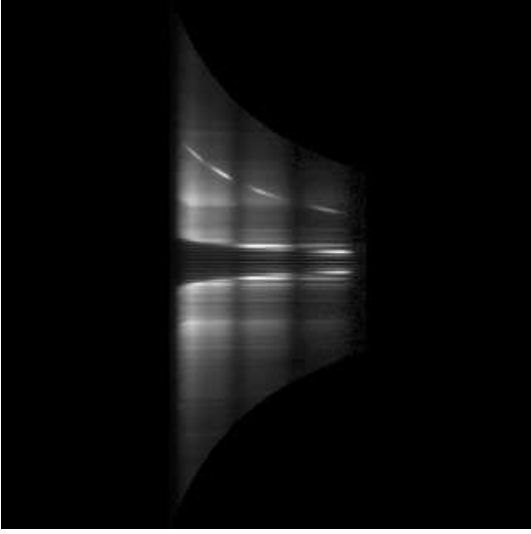
Fig. 2. Same spectrum as Fig. 1 where each column has been rescaled according to its corresponding central wavelength to correct for the spectral dependence of the speckles. The speckles are now along straight horizontal lines, and the planet follows a 1/\lambda law. The displaying scale is the same as in Fig. 1.
