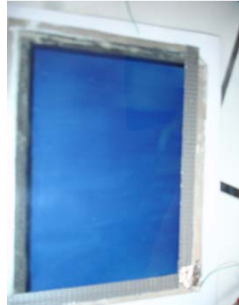
a) Bleached and colored states after 2 600 cycles between +1.0V and -1.3V
