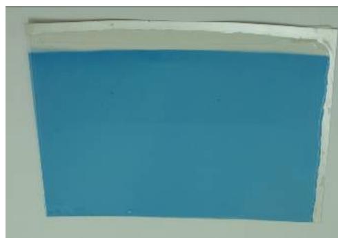
Figure IV.5 : Prussian Blue deposited on ITO/PET at 90% of PEDOT capacity
