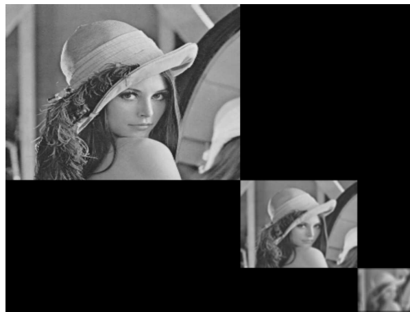
(b) Pyramid obtained with a mean filter having applied on a window of variable size
