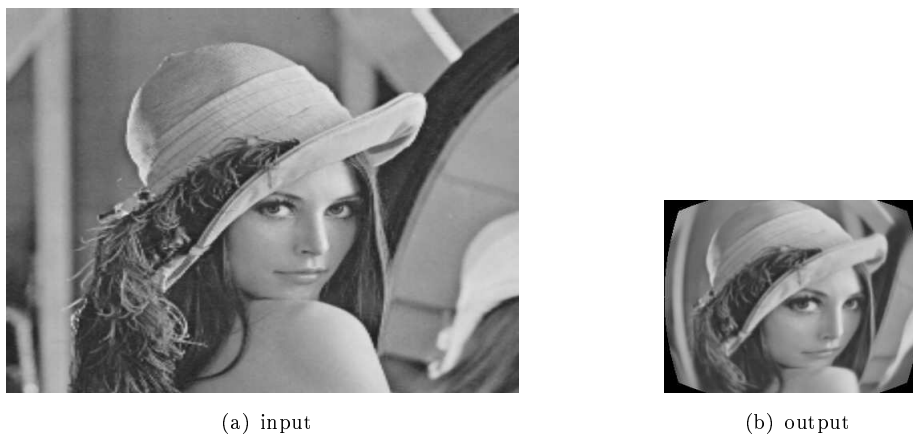
Figure 10.1: Example of an input and output images for a space-variant low-pass followed by a LOG sampling
