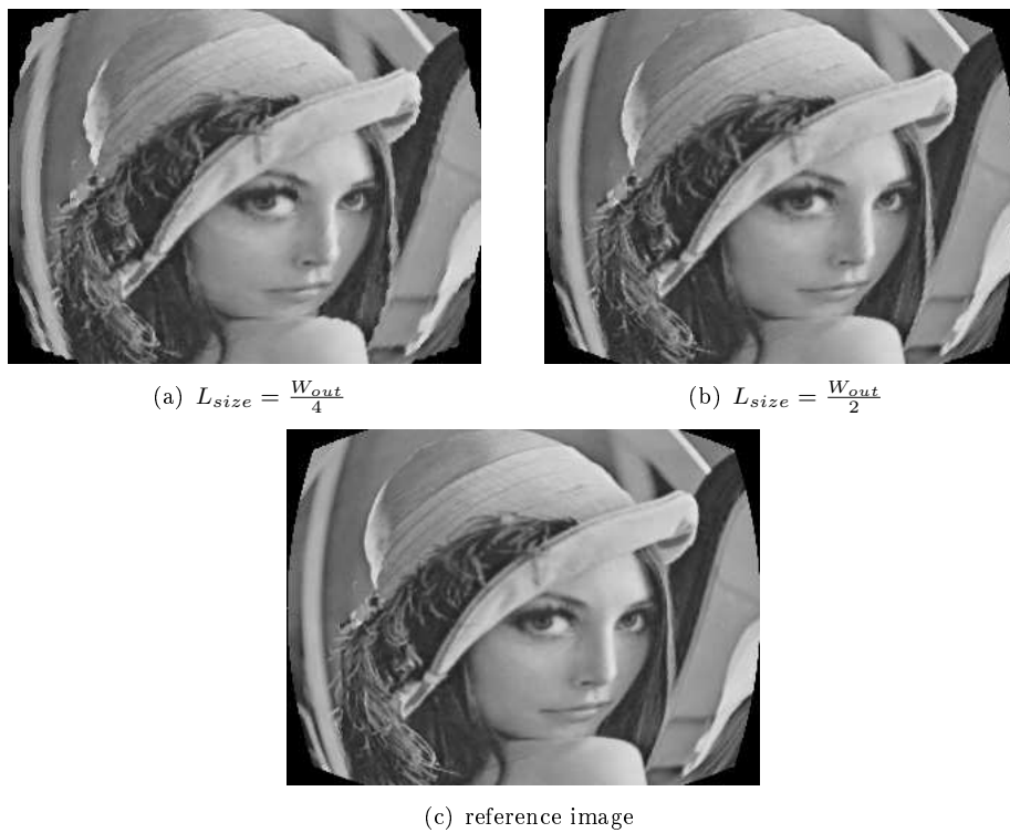
Figure B.4: Output of an approximated LOG sampling applied to a VGA image and using different LUT size
