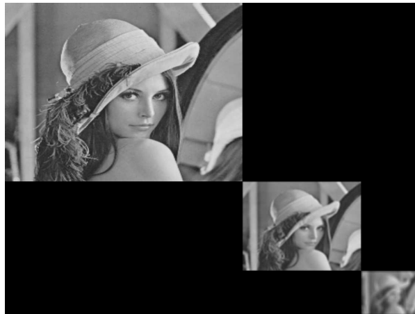
Figure 10.2: Example of a pyramid with 3 levels and constructed with a low-pass having a window size variable with the number of level
