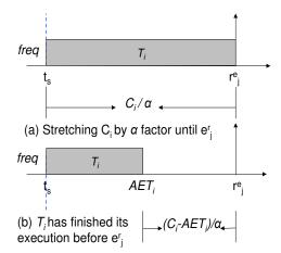
FIGURE 3.11: Idle time on the processor
