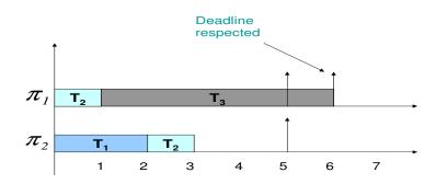
FIGURE 4.2: EDZL removes dhall's effect
