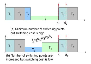
FIGURE 3.13: Gradual increase in frequency of the processor
