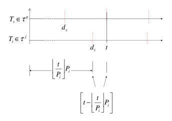
FIGURE 5.11: Maximum demand of tasks on processor
