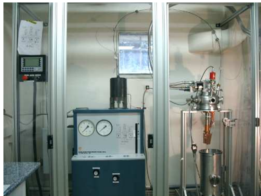
Figure 1. Picture of the high-pressure and low-temperature setup. The black cylinder in the middle of the picture is the third pressure stage that goes up to 1.5 GPa. On top of it is the capillary tube, which brings the pressure to the cell, which itself is fixed to the cold head of the cryostat on the right. The screen on the left is for pressure command.
