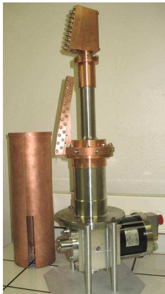
Figure 3. Picture of the cold head with the copper parts designed to tight and cool down the cell (2nd stage, on top) and the capillary tube (1st stage, on bottom). On the left of the cold head is the thermal screen that is then fixed to the 1st stage. See text for details.
