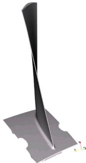
Figure 3.11: Geometry of the booster blade
