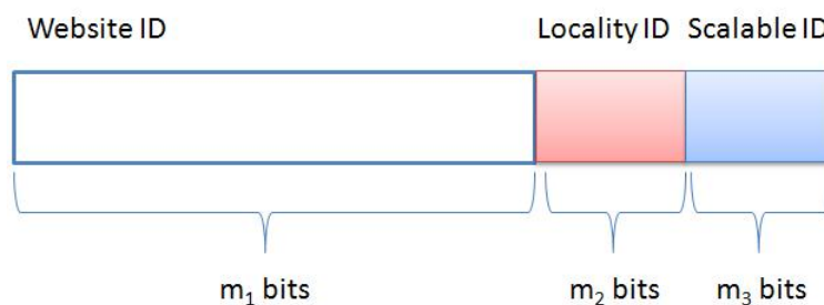
Figure 4.1: Peer ID structure in D-ring of PetalUp-CDN.
