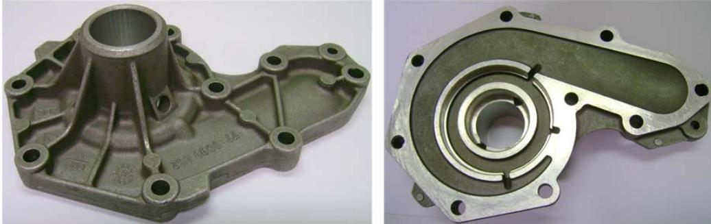
Figure 6-4: Automotive water pump cover
