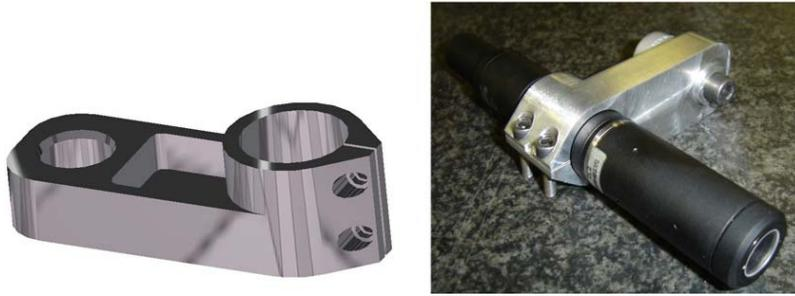
Figure 6-2: The component to install the STIL pen on CMM arm
