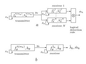
Fig. 2.5 – Parameter modulation
