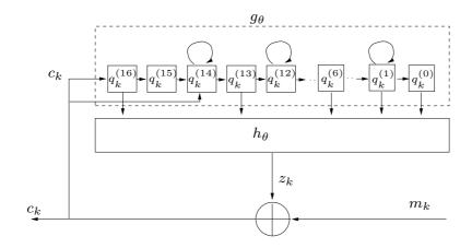
Fig. 4.4 – Block diagram of SSS
