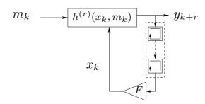
Fig. 4.1 – Self-synchronizing Message Embedded Stream Cipher
