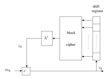
Fig. 4.2 – Block cipher in CFB mode
