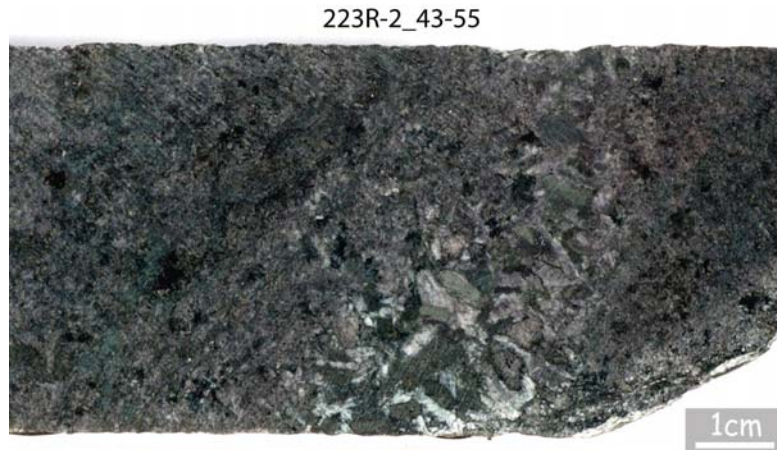
Figure II-10: Photograph of core 223R-2_43-55 from IODP Hole 1256D (zone 4). Fine and coarse grained gabbroic domains are observed (image is from the data base of Expedition 312 in Teagle et al., 2006).
