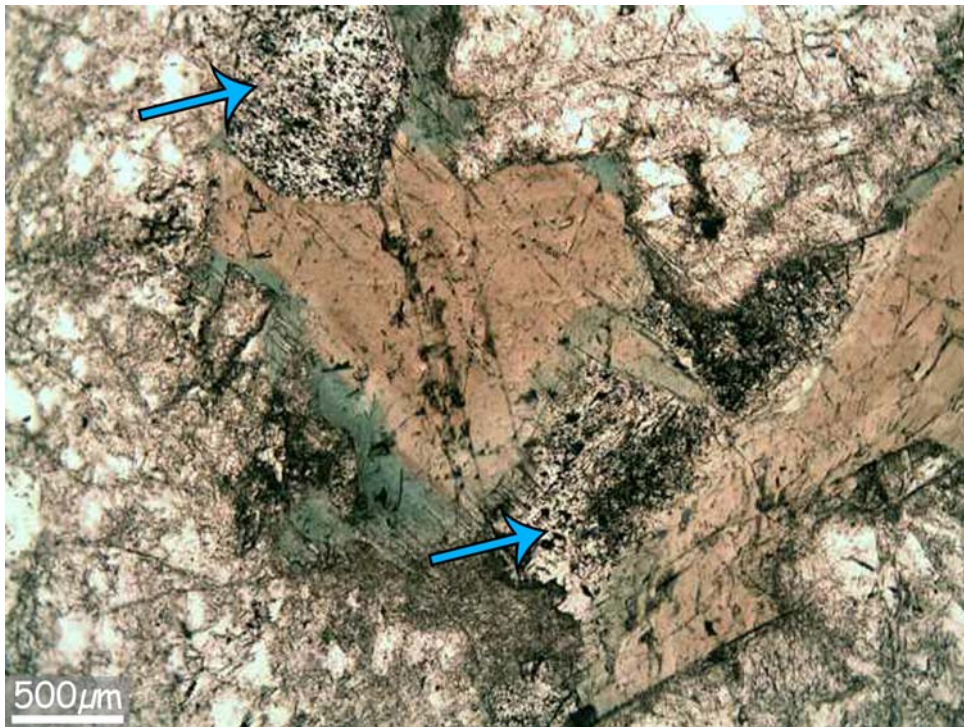
Figure III-21: Microphotograph of an isotropic gabbro sample (sample 08OLC3b) showing the retrograde evolution from the magmatic stage to the green schist facies conditions (plane-polarized light). Altered clinopyroxenes (blue arrows) attest to the magmatic conditions, brown amphibole attests to the amphibolite facies conditions and green amphibole attests to the green schist / amphibolite facies conditions.
