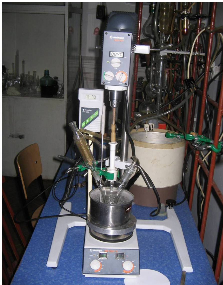
Fig. 4-4. Installation used for suspension polymerisation.
