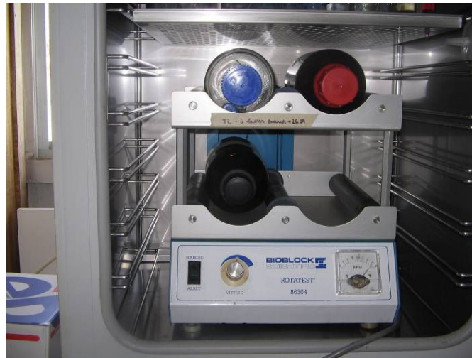
Fig. 6-18. Installation for microbeads homogenous turning – calcification tests.
