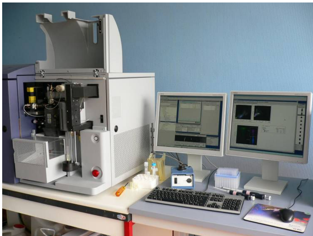
Fig. 6-29. BD FACS Aria Flow Cytometer
