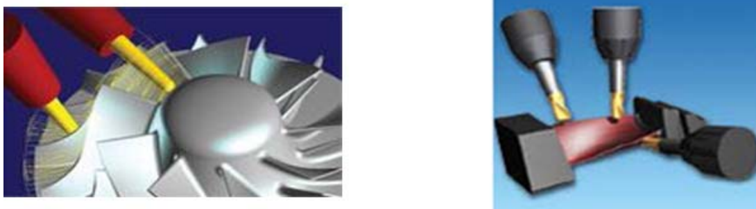
Figure 4. Usinage 5 axes continus [Livre TopSolid-Cam]
