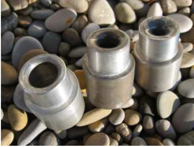
FIGURE 3.8: (a) Photo of the three removable blockage sections constructed for the experimental rig. From left to right, the blockages correspond to b = 0.50 , 0.75 and 0.90 . A small portion of the curve of the stenoses inside each section can be discerned. (b) Schematic of the removable blockage section.
