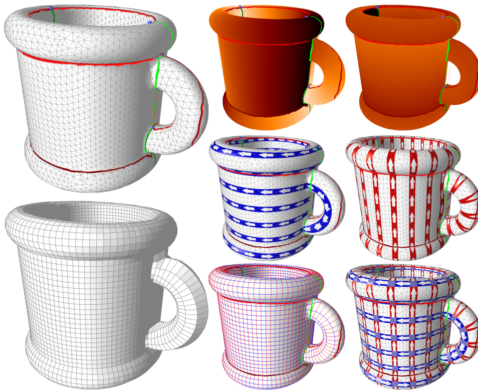
Figure 2.36: Genus-1 model. Left: input triangle surface mesh with singularity graph covering the homology generators, and the final quadrangle tiling. Right, top: u, v . Right, middle: du and dv . Right, bottom: iso-contouring lines, and du - dv .
