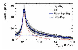
Figure 6.33: Fit to the signal plus background using *Kernel Estimation* for eeX-channel with polarization mode  $e_R^-e_L^+$  in MD analysis, with Bremsstrahlung recovery.
