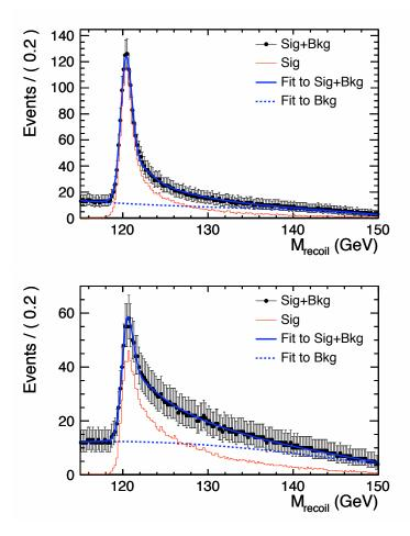
Figure 6.22: Fit to the signal plus background using *GPET Function* of  $\mu\mu X$  (top) and eeX (bottom) channels with polarization mode  $e_{\rm L}^-e_{\rm R}^+$  in MD analysis.
