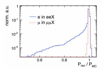
Figure 3.9: Distributions of the ratio between reconstructed momentum and Monte-Carlo truth for electrons and muons, using the Higgs-strahlung samples with  $Z \to e^+e^$ and  $Z \to \mu^+\mu^-$ , respectively.
