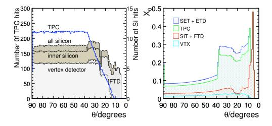
Figure 3.4: Left: Average number of hits for simulated charged particle tracks as a function of polar angle[29]. Right: Average total radiation length of the material in the tracking detectors as a function of polar angle[29].
