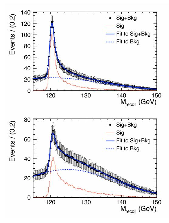
Figure D.9: Fit to the signal plus background using *Physics Motivated Function* of  $\mu\mu X$  (top) and eeX (bottom) channels with polarization mode  $e_{\rm L}^-e_{\rm R}^+$ , in MI analysis.
