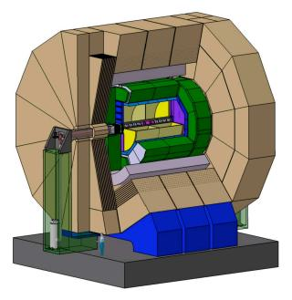
Figure 3.3: View of the ILD detector concept[29].
