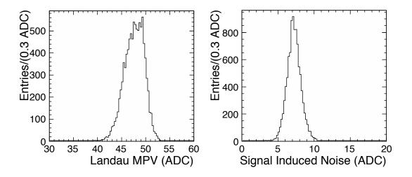
Figure 5.9: Left: Distribution of Landau MPV (calibration constant) with each entry representing a pad, with a mean of  $47.61 \pm 0.02$  ADC counts and a RMS of  $2.06 \pm 0.01$  ADC counts. Right: Distribution of signal induced noise with each entry representing a pad, with a mean of  $7.22 \pm 0.01$  ADC counts and a RMS of  $1.00 \pm 0.01$  ADC counts.
