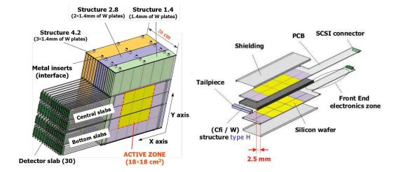
Figure 4.1: Left: Schematic view of the SiW prototype. Right: Schematic diagram showing the components of a detector slab[32].
