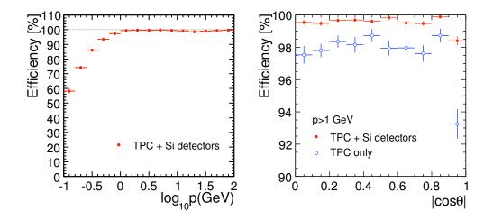
Figure 3.6: Tracking Efficiency as a function for  $t\bar{t} \rightarrow 6$  jets at 500GeV plotted against momentum (left) and  $\cos \theta$  (right). Efficiencies are plotted with respect to MC tracks which leave at least 4 hits in the tracking detectors including decays and  $V^{0}s[29]$ .
