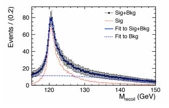
Figure 6.32: Fit to the signal plus background using *Kernel Estimation* for eeX-channel with polarization mode  $e_{\rm L}^-e_{\rm R}^+$  in MD analysis, with Bremsstrahlung recovery.
