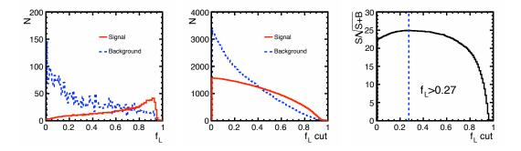
Figure A.6: Same as Figure A.1, but for the eeX-channel with polarization mode  $e_{\rm L}^-e_{\rm R}^+$  in the MD Analysis.
