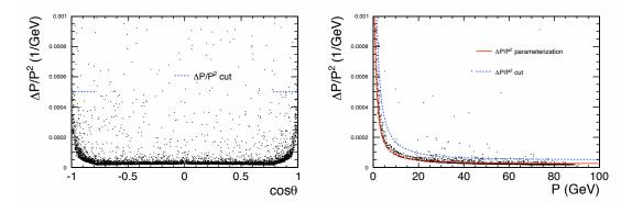
Figure 6.3: 2D  $\Delta P/P^2$  distribution vs.  $\cos\theta$  (left) and  $\Delta P/P^2$  distribution vs. track momentum (right) of electron candidates decayed from Z<sup>0</sup> of Higgs-strahlung process.
