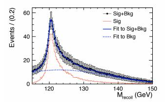
Figure 6.31: Fit to the signal plus background using *Kernel Estimation* for eeX-channel with polarization mode  $e_{R}^{-}e_{L}^{+}$  in MI analysis, with Bremsstrahlung recovery.
