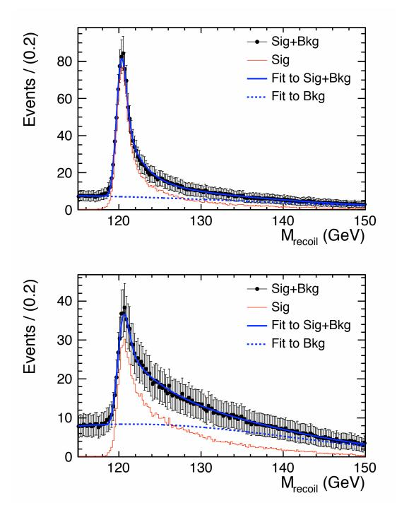
Figure D.12: Fit to the signal plus background using *Physics Motivated Function* of  $\mu\mu X$  (top) and eeX (bottom) channels with polarization mode  $e_{\rm R}^-e_{\rm L}^+$ , in MD analysis.
