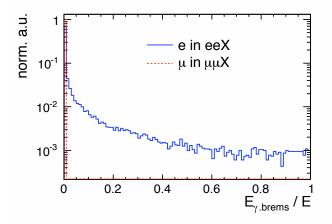
Figure 3.8: Distributions of the fraction of Bremsstrahlung energy loss for electrons and muons before entering TPC, using the Higgs-strahlung samples with  $Z \to e^+e^$ and  $Z \to \mu^+\mu^-$ , respectively.
