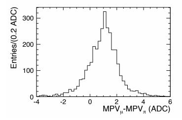
Figure 5.11: Differences of the calibration constants for each pad, between that obtained from muons with  $20 \times 20$  trigger and from pions with  $10 \times 10$  ÅČerenkov, with a mean of  $0.97 \pm 0.02$  ADC counts and a RMS of  $1.19 \pm 0.02$  ADC counts.
