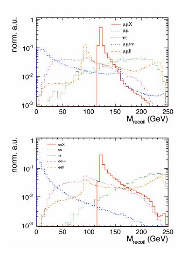
Figure 6.9:  $M_{\text{recoil}}$  distributions of  $\mu\mu X$  (top) and eeX (bottom), and of their corresponding backgrounds.
