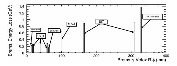
Figure 3.11: Mean Bremsstrahlung energy loss as a function of the Bremsstrahlung photon vertex in the barrel region of the ILD detector, for electrons in the Higgs-strahlung sample with  $Z \rightarrow e^+e^-$ . The vertices correspond to the positions of the detector components as labeled, with the mean energy loss proportional to the amount of material.
