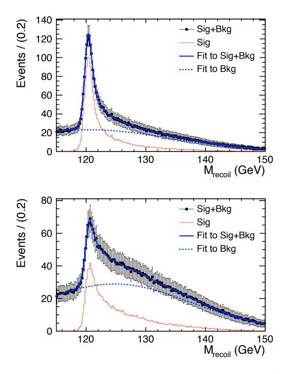
Figure D.5: Fit to the signal plus background using *Kernel Estimation* of  $\mu\mu X$  (top) and eeX (bottom) channels with polarization mode  $e_{\rm L}^-e_{\rm R}^+$ , in MI analysis.
