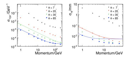
Figure 3.5: Left: Transverse momentum resolution for muons plotted versus polar angle for four different simulated muon momenta. The lines show  $\sigma_{1/p_T} = 2 \times 10^{-5} \oplus 1 \times 10^{-3}/(p_T \sin \theta)$  for  $\theta = 30^{\circ}$  (green) and  $\theta = 85^{\circ}$  (blue)[29]. Right: Impact parameter resolution for muons versus polar angle for four different simulated muon momenta[29].
