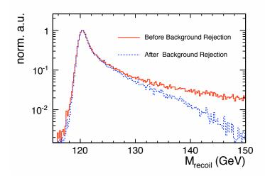
Figure 6.20:  $M_{\text{recoil}}$  distribution of Signal *before and after background rejection*. Maximum of the distributions are normalized to be *one*. Illustration using MI analysis,  $\mu\mu X$  channel with polarization mode  $e_{\rm L}^-e_{\rm R}^+$ .
