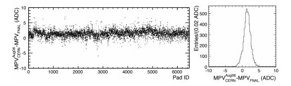
Figure 5.15: Left: Difference of the calibration constants between October 2006 CERN runs and 2008 FNAL runs as a function of pad index (defined in Equation 5.2). Right: Distribution of the difference of each pad, with a mean of  $1.42 \pm 0.01$  ADC counts and a RMS of  $1.08 \pm 0.01$  ADC counts.
