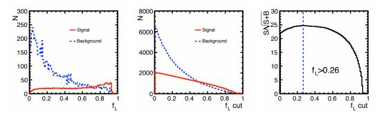
Figure 6.17: The distributions of the Likelihood Fraction  $f_L$  (left), the number of remaining events versus the cut on  $f_L$  (middle), and the significance versus  $f_L$  cuts (right). The distributions are shown for the  $\mu\mu X$ -channel with polarization mode  $e_L^- e_R^+$  in the MI Analysis.
