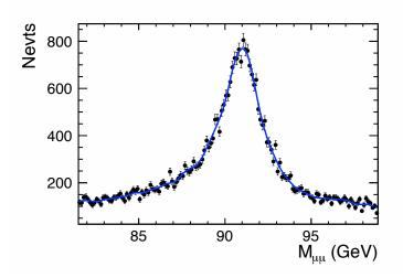
Figure 6.34: Fit of the *Invariant Mass* of the  $Z \to \mu^+ \mu^-$  in the ZZ process using *Kernel Estimation*, with polarization mode  $e_L^- e_R^+$ . An accuracy of 13 MeV is obtained for the invariant mass measurement.
