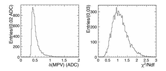
Figure 5.7: Left: Distribution of the statistical error of fitted Landau MPV for each pad, with a mean of  $0.516\pm0.002$  ADC counts and a RMS of  $0.173\pm0.001$  ADC counts. Right: Distribution of  $\chi^2/Ndf$  for each pad of the fit to the hit energy spectrum, with a mean of  $1.139\pm0.004$ , with a RMS of  $0.394\pm0.003$ .
