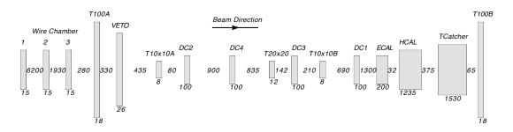
Figure 5.2: Beam line setup of the beam test at FNAL in 2008. The Čerenkov detector in the up stream, which is not drawn in this figure. All distances and dimensions are in mm.
