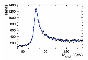
Figure 6.35: Fit of the *Recoil Mass* to the  $Z \to \mu^+ \mu^-$  in the ZZ process using *Kernel Estimation*, with polarization mode  $e_L^- e_R^+$ . An accuracy of 28 MeV is obtained for the Z recoil mass measurement.
