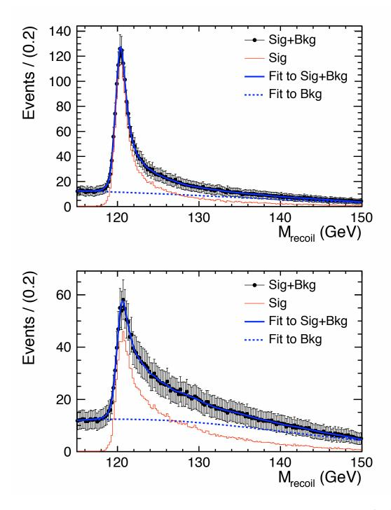
Figure D.7: Fit to the signal plus background using *Kernel Estimation* of  $\mu\mu X$  (top) and eeX (bottom) channels with polarization mode  $e_{\rm L}^-e_{\rm R}^+$ , in MD analysis.
