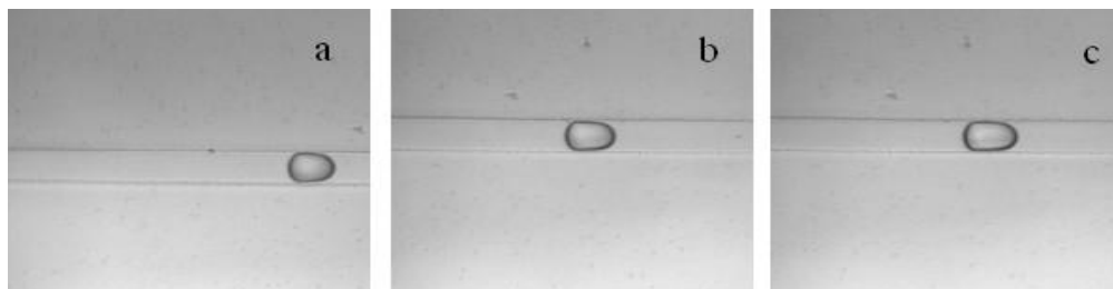
Débits calibrés : a) Q_c :20 \mu\text{L}/\text{min} , Q_l :4 \mu\text{L}/\text{min} ; b) Q_c :20 \mu\text{L}/\text{min} , Q_l :5 \mu\text{L}/\text{min} ; c) Q_c :20 \mu\text{L}/\text{min} , Q_l :6 \mu\text{L}/\text{min} .
