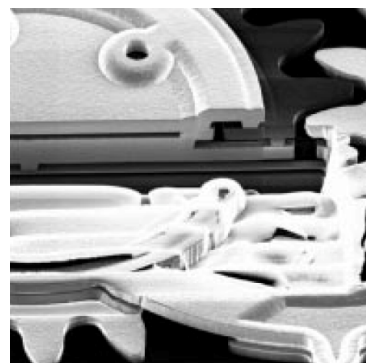
Figure 1-5 Examples fabricated by bulk micromachining and surface micromachining technologies.
