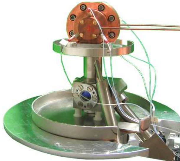
Figure 8: The HORACE clock: the cooling and the interrogation take place in the microwave cavity (copper block on top), which is part of a UHV chamber. The laser light is coupled by multimode glass fibers (green cables), the microwave is coupled by waveguides (rods connected to the cavity). Image courtesy of F.X. Esnault.
