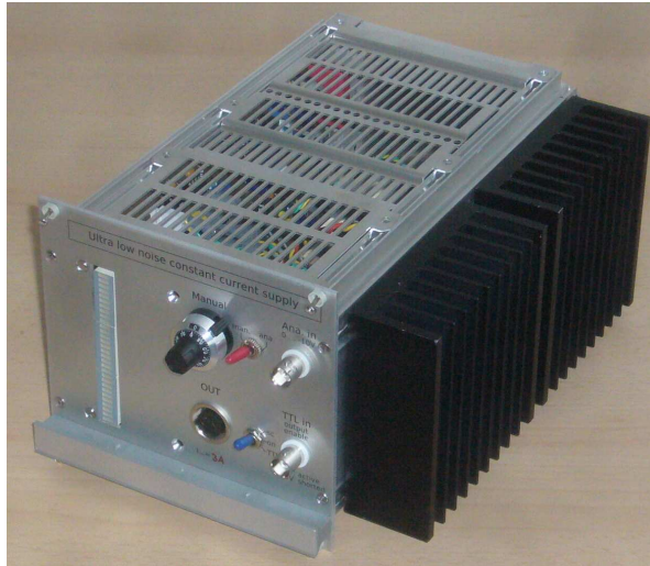
Figure 61: The housing of the current source. All power-carrying components are mounted on separated heatsinks (right).
