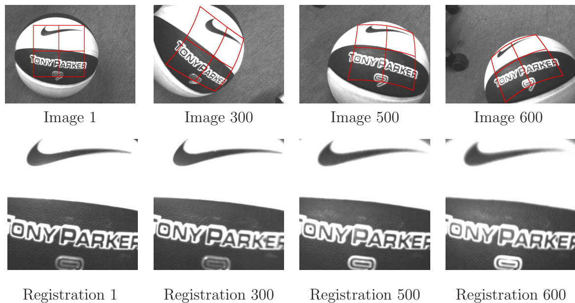
FIG. 3.7 – Image registration with an uncalibrated pinhole camera in a sequence of 600 images. The top row shows the (4 \times 4) regular grid used to align the area of interest in the sequence. The bottom row shows the area of interest registered with respect to the template.
