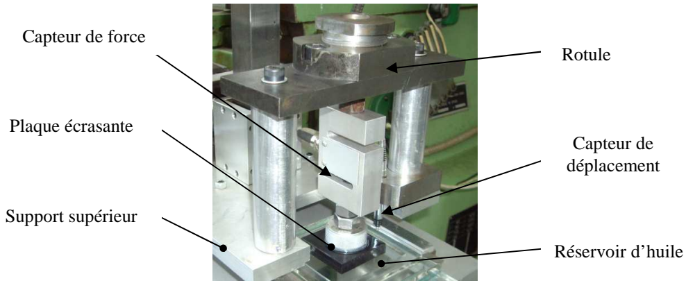
Figure III.2: Instrumentation du banc
