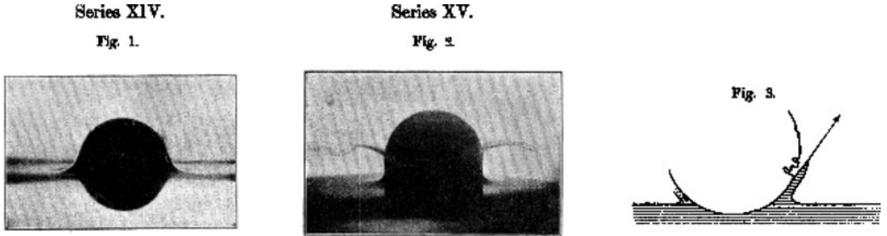
FIGURE 6. Figures extracted from Worthington & Cole (1900): (a) impact in water of a smooth sphere (b) impact at the same conditions of a rough sphere (c) proposed mechanism for the influence of the roughness.
