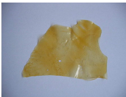
Figure 9 : Membrane made of hydrolyzed poly(VDF-ter-CTFE-ter-PFSVE) terpolymer.
