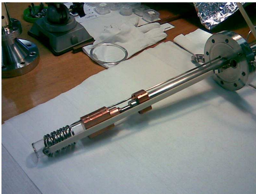
Fig. 3.1: Image of the rf oxygen plasma source used to grow our epitaxial oxide films. At the end of the source one can distinguish the radio frequency quartz cavity containing one single effusion hole to release the oxygen atoms.
