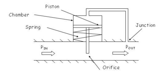
Figure 73: Pressure regulator schematic representation [Bashkar and Nigam, 1990]
