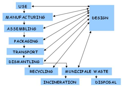
Figure 5: The physical design life cycle model
