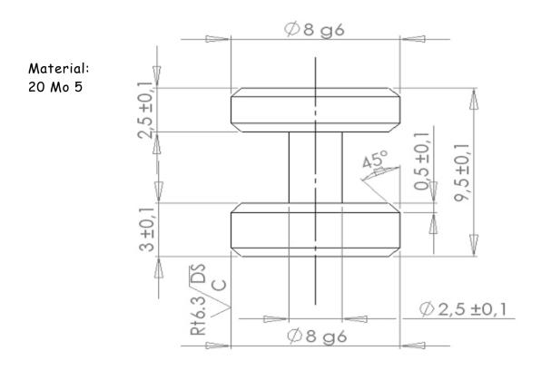
Figure 76: Drawing of the piston of a pressure regulator with the fundamental functional dimensions and the separation variables
