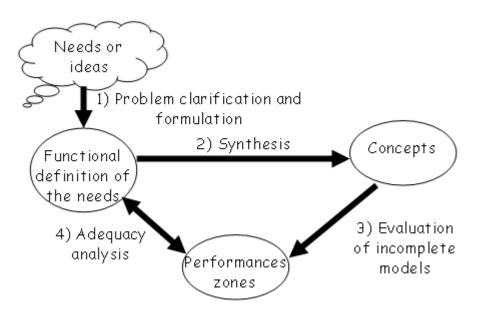
Figure 1: The Conceptual design process [Yannou, 2001]
