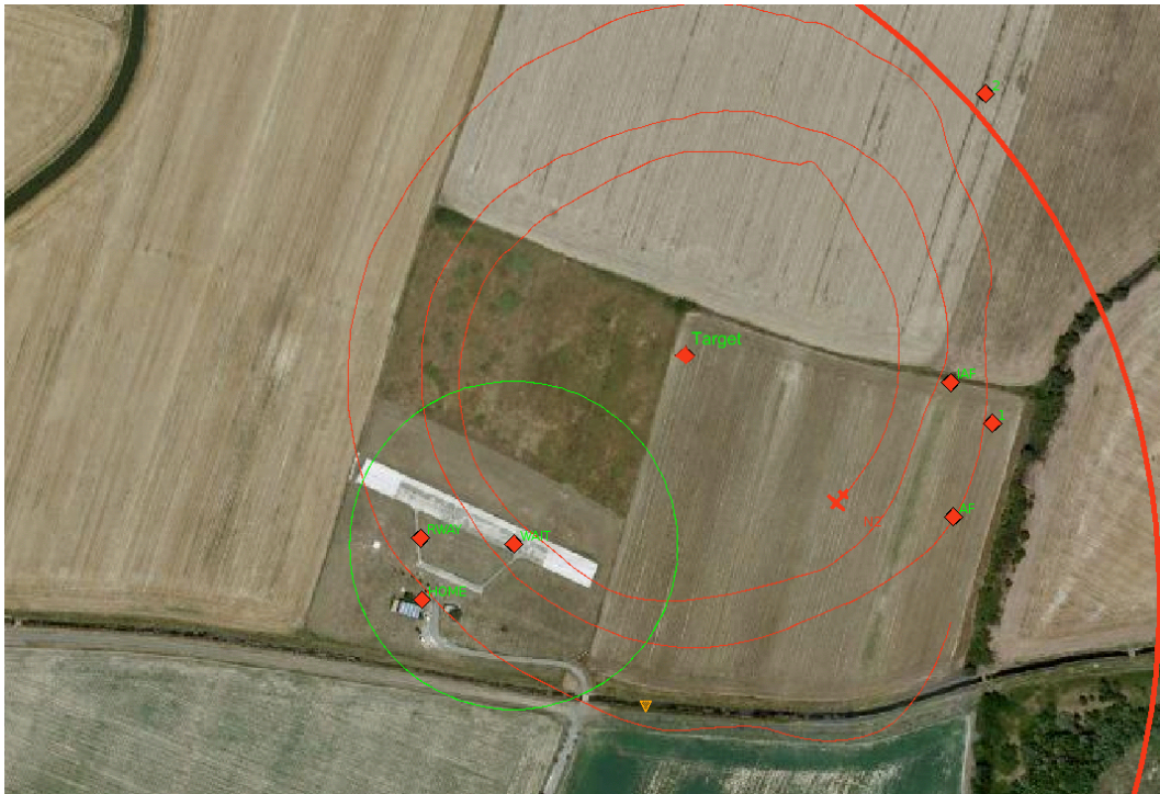
Figure 4.12: A static target tracking trajectory over our test field. The target is static sitting in the middle of the field. The red dots at the right part are rendez vous point that help initiate the experiment.
