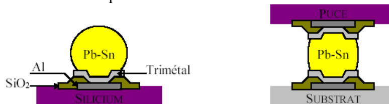
Figure 2: Technologie Flip Chip IBM [Dav06]
