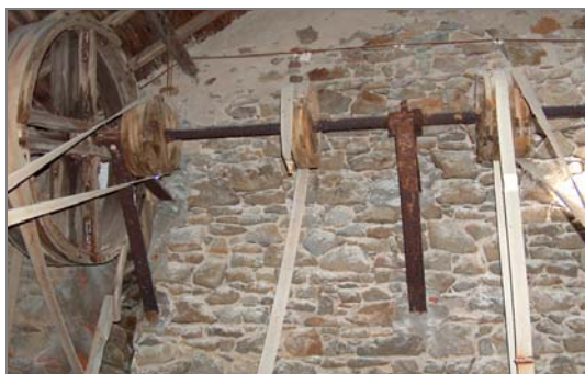
Figure 145 : PHOTO, ARBRE PRINCIPAL
