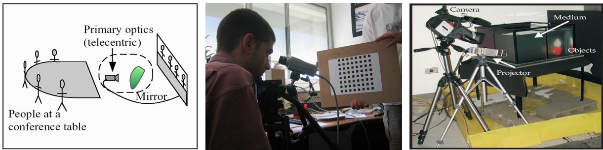
Figure 1.5: Three interesting scenarios showing the importance of generic imaging models. Left: Designing a catadioptric configuration (using a mirror) for custom viewing of a scene [109]. Middle: Shape reconstruction of the cornea of the eye by capturing the image of the scene reflected by the cornea [43]. Right: Camera looking at a scattering media to study structured light algorithms [68].
