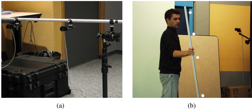
Figure 4.2: (a): Partial view of a 30-camera setup. (b): The calibration data are gathered by moving a one-dimensional object in the common field of view of the cameras.
