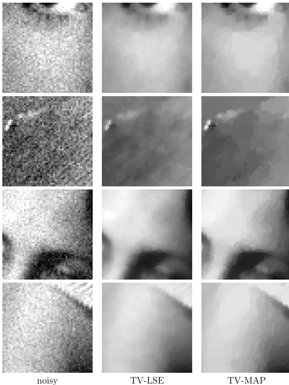
Figure 4.29: Reduction of the staircasing effect. We take the images of Figures 1.4 and 1.5, and experimentally check that TV-LSE does not create staircasing artefacts. The left column shows zooms of Lena and Barbara images with Gaussian white noise added (s.d. 10). The middle column shows the corresponding TV-LSE denoised images ((\lambda, \sigma) = (40, 10)) , while the right column shows the TV-MAP denoised images corresponding to equivalent level of denoising (from top to bottom: \lambda_{MAP} = 25.6 , \lambda_{MAP} = 20.3 , \lambda_{MAP} = 29.0 , \lambda_{MAP} = 26.9 ). Staircasing effect is huge in TV-MAP but does not occur in TV-LSE.
