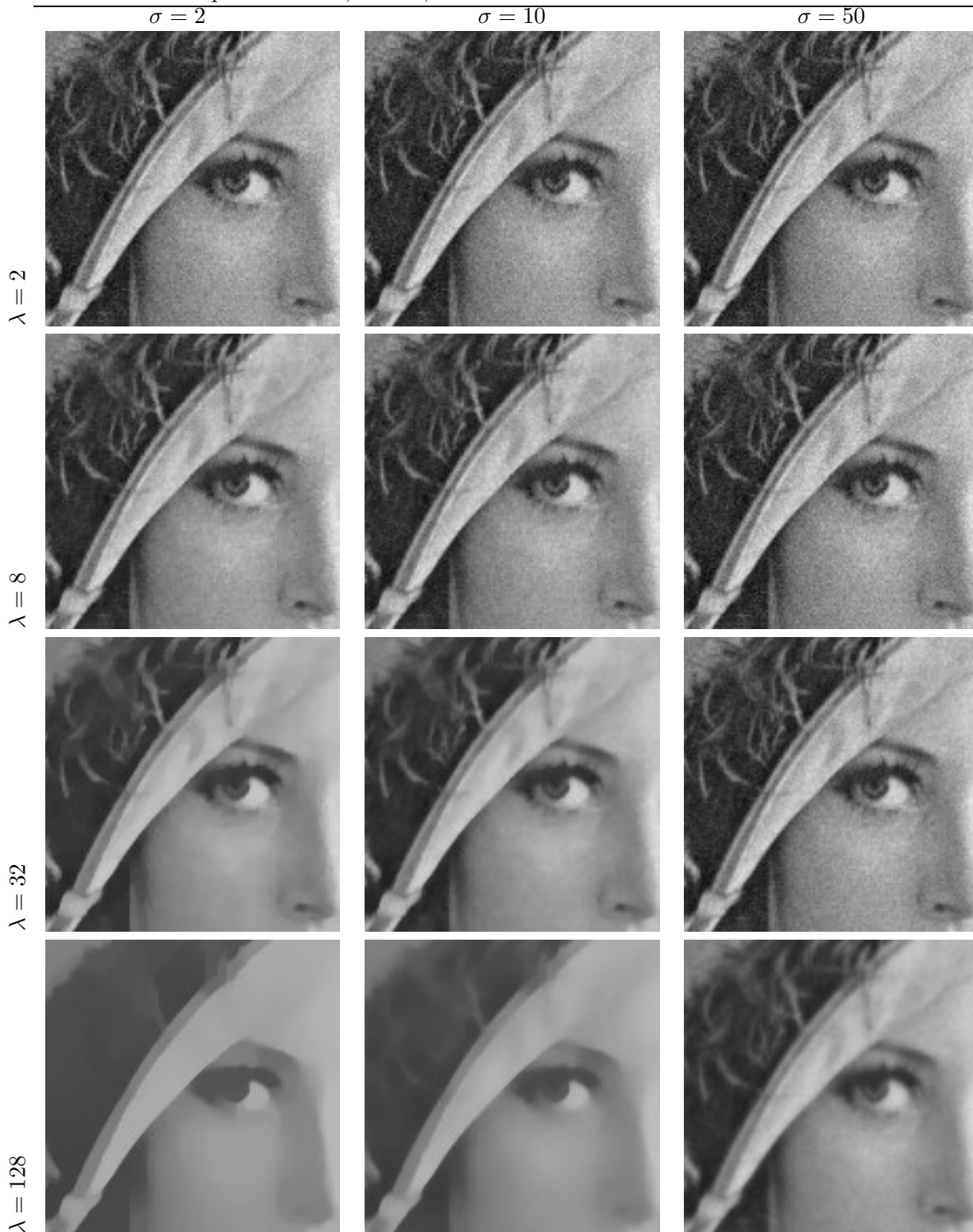
Figure 4.4: Influence of the parameters \lambda and \sigma on \hat{u}_{LSE}(\lambda, \sigma) . The Lena image was corrupted by a Gaussian white noise with s.d. 10 (see Figure 4.1, top-left image), and denoised using the fully automatic TV-LSE algorithm (optimal scaling, automatic burn-in, and \varepsilon = 1 ). A column considered alone ( \sigma fixed) starts on top with a rather noisy image, and is more regular as we get down (as \lambda increases), with preserved boundaries, regularized smooth regions (no staircasing visible) and erased texture. A row considered alone ( \lambda fixed) starts on the left with a regularized image which is not far from \hat{u}_{MAP}(\lambda) (because \hat{u}_{LSE}(\lambda, \sigma) converges to \hat{u}_{MAP}(\lambda) when \sigma \rightarrow 0 ), and details of the texture and then noise appear when scrolling to the right, hence coming closer to the noisy image (the input). These observations are consistent with the table of Figure 3.2. SNR are given Figure 4.7.
