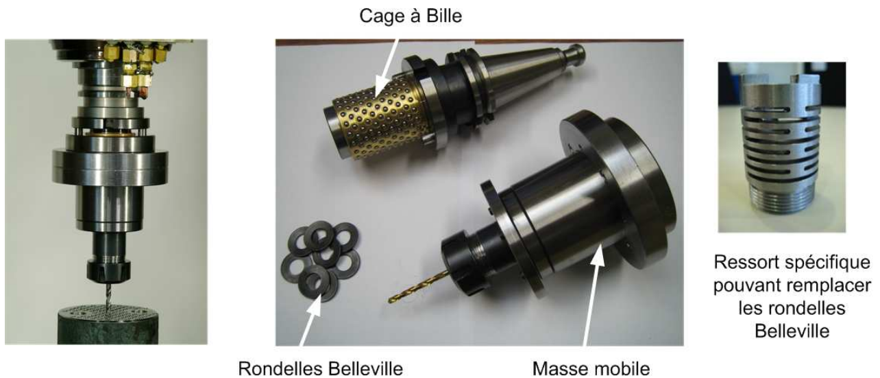
Figure III.6: Composition de la tête N°2.
