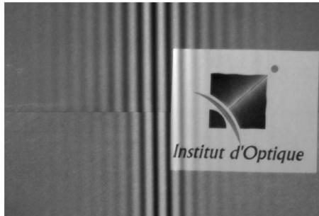
Fig. 2 Image showing fringes superimposed on the field of view. The upper part of the background is red when the lower part is blue.
