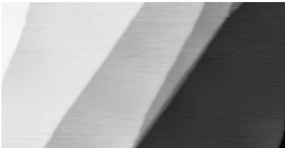
Figure 3.14: Large scale image of the clean Cu(111) surface (STM image size 190 \times 100 \text{ nm}^2 , I=0.2 \text{ nA} , V=-40 \text{ mV} ).
