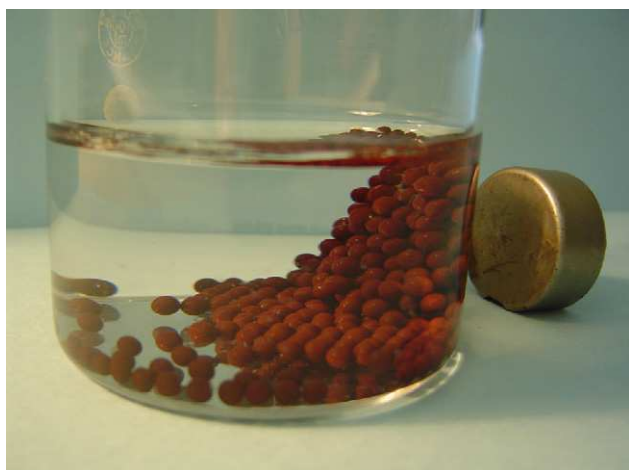
Fig. 1 – Photograph of magnetic alginate beads attracted by a magnet.
