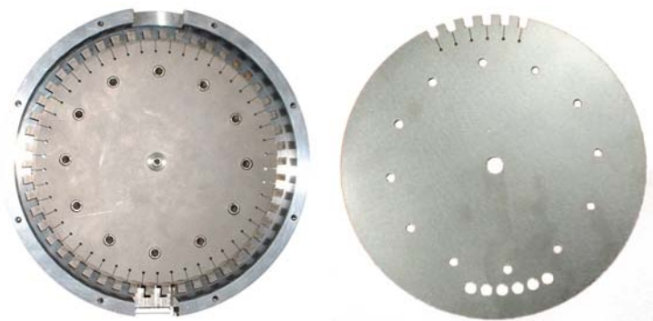
Fig. I.13: The fifty-tooth wheel ( \varnothing 185 mm, left) and the six-tooth wheel ( \varnothing 185 mm, right)
