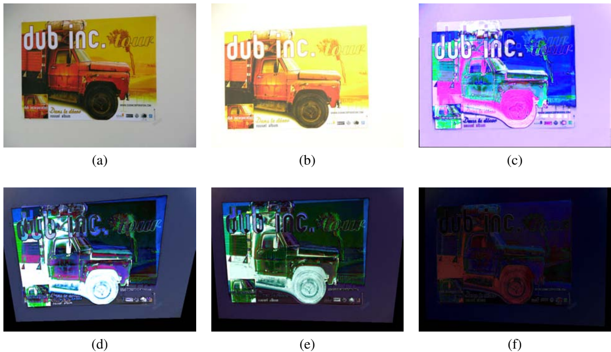
Figure 6.1: Paper (PAMI'08) – Groupwise Geometric and Photometric Direct Image Registration . Example of pixel-based geometric and photometric image registration. The two images were registered using our dual inverse compositional algorithm . (a) and (b) show the two original images. The lighting is different in intensity and color. (c) – (f) are a selection of difference images through the registration process, from the start to convergence.
