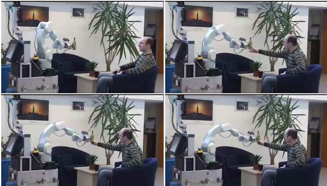
Figure 5.18: When the actions of a “hand over an object” task are run sequentially, the robot only releases the object when the arm reaches its position. For a person who wants to take the object earlier, this behavior causes discomfort in the interaction.
