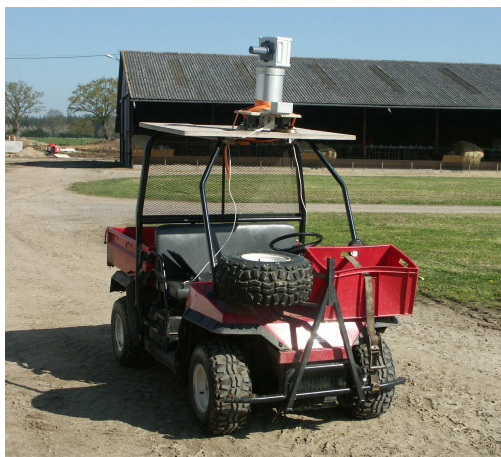
Figure 5.12 – L'antenne directive mobile
