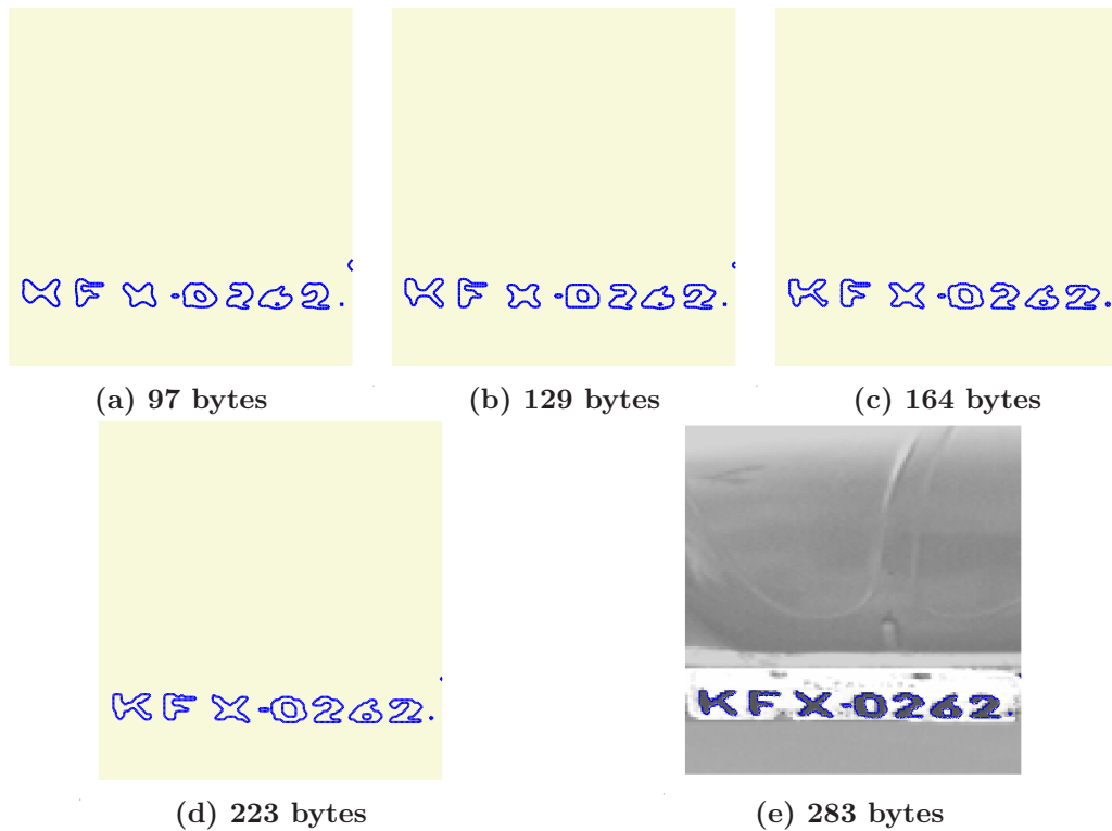
Figure V.21: Progressive compression of a car number plate (with enhanced contrast), topology controlled: direct encoding (173 bytes) and progressive encoding (283 bytes) both with good compression ratio.
