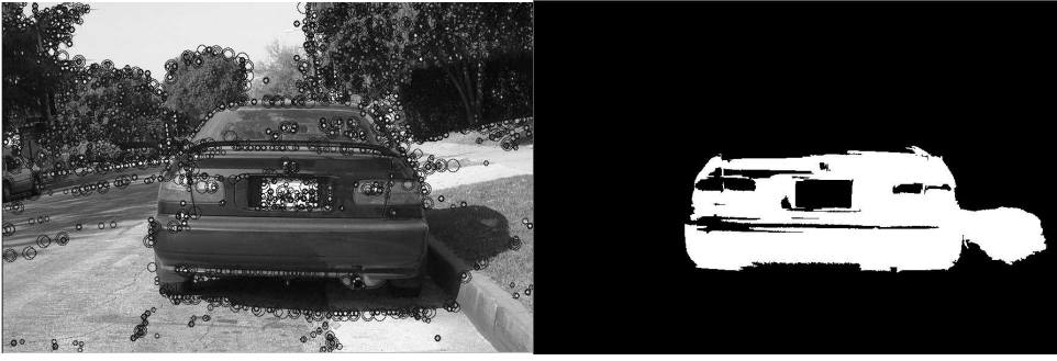
Figure 7.8: Example of SIFT features computed on an image containing a car. On the right, the associated segmented image (after region selection). The resulting mask is used to filter the key-points detected in the background: any key-point which is not in the area resulting from segmentation is not taken into account by visual detection.
