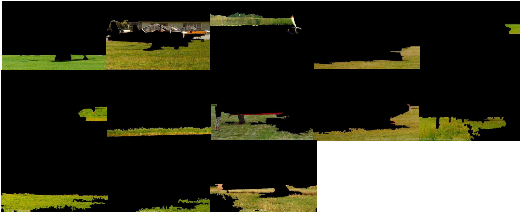
Figure 7.5: A set of regions obtained by a weakly-supervised approach ( a = Hue ). This cluster is labeled with the visual concept Green . All these regions result from automatic segmentation of the image training set.
