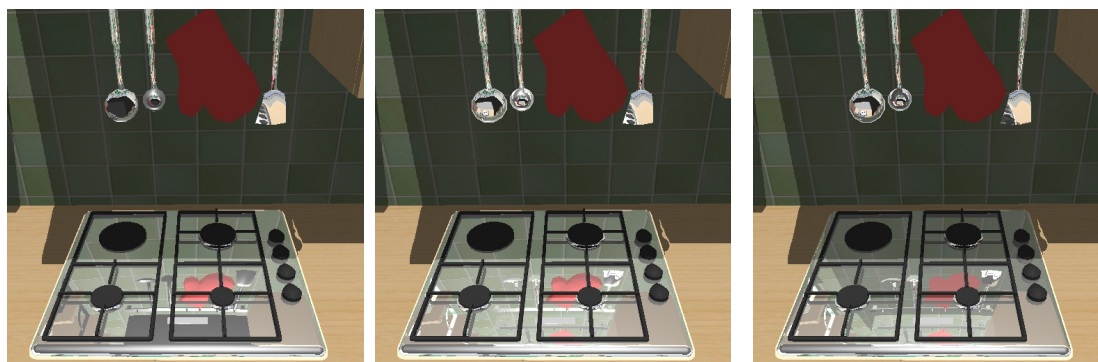
(a) 1 specular reflection (302 ms). (b) 2 specular reflections (674 ms). (c) 2 specular refl.+shadows (993 ms).
