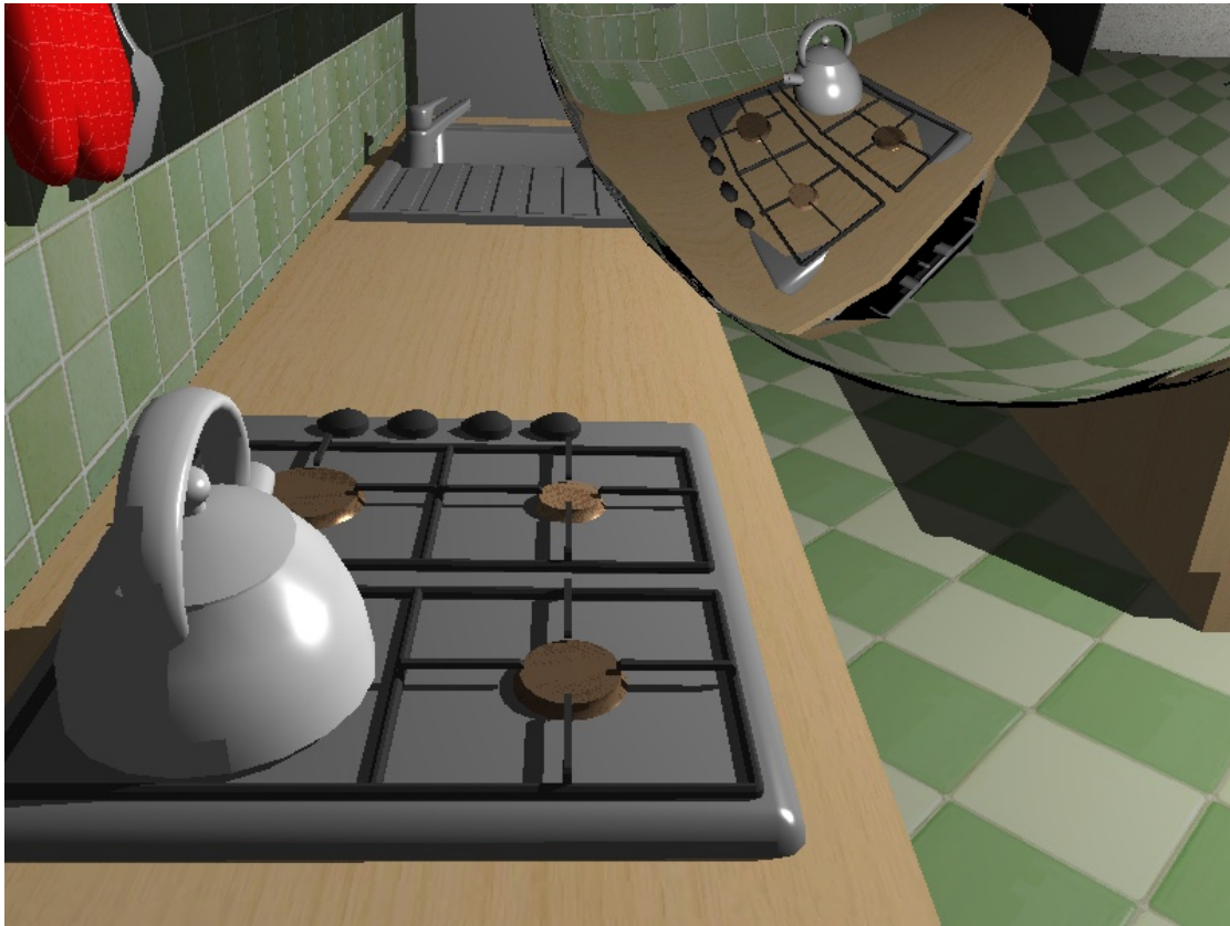
Figure 2.18: Example of Z-fighting when a small object is layered on top of a larger object.
