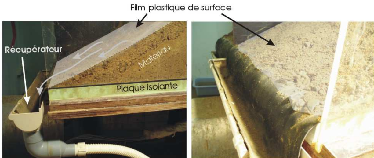
Water and eroded material recovery system.
