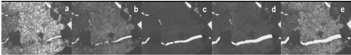
Figure II.10 – Transition \alpha \rightarrow \beta de AgI ( P = 2,96 kbar – T = 100^{\circ}\text{C} )
