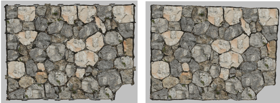
Figure 4.22 Left: A generated structure before the junction correction process. Right: The same structure after the correction process.
