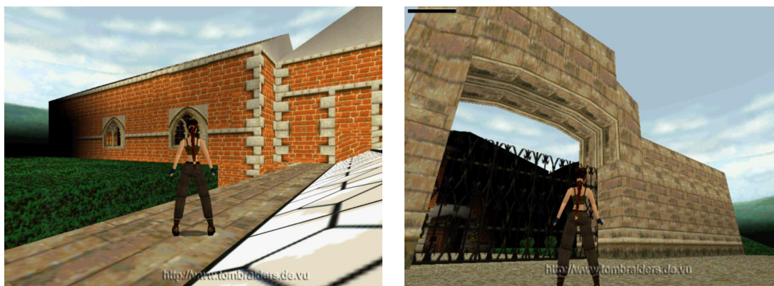
Figure 1.2 Texture mapping structured textures often exhibits annoying artefacts: parametrization problems, structure repetitions, limited resolution. (Images from [tom])
