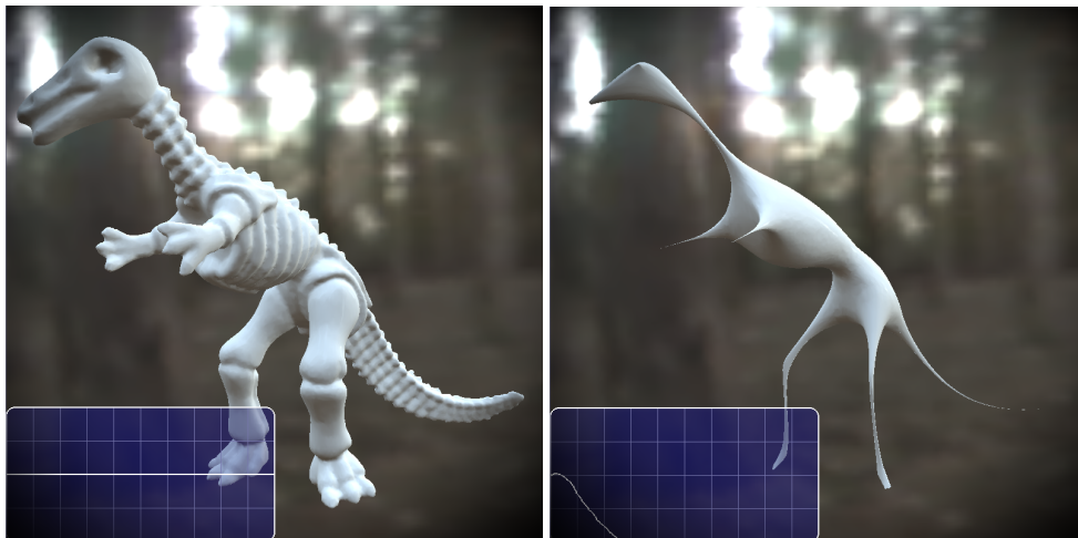
FIG. 5.11 – Very intense smoothing (right) of a dinosaur model (left) generates counterintuitive spikes.
