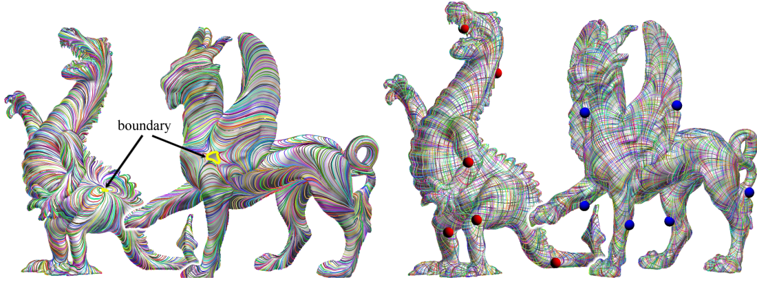
FIG. 10.3 – Left : removing geometric influence on a topological disk (left) and a genus 2 surface with a border (right). Right : if no geometric influence is wanted, the algorithm evenly distributes singularities on the surface : 8 singularities of index 1/4 on topological sphere (left), and 8 singularities of index -1/4 on genus two surface (right).
