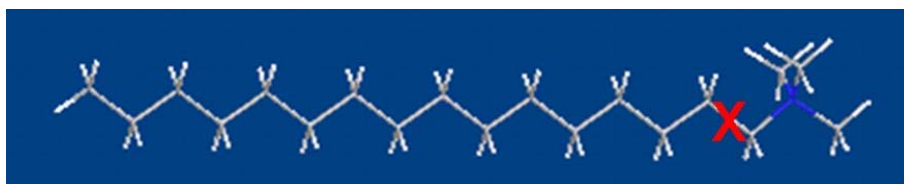
Scheme 5.3 Cetyltrimethylammonium ion (CTA + ) with a longer tail used as template reagent in [S + I] type synthetic pathway of MCM-41 silica.
